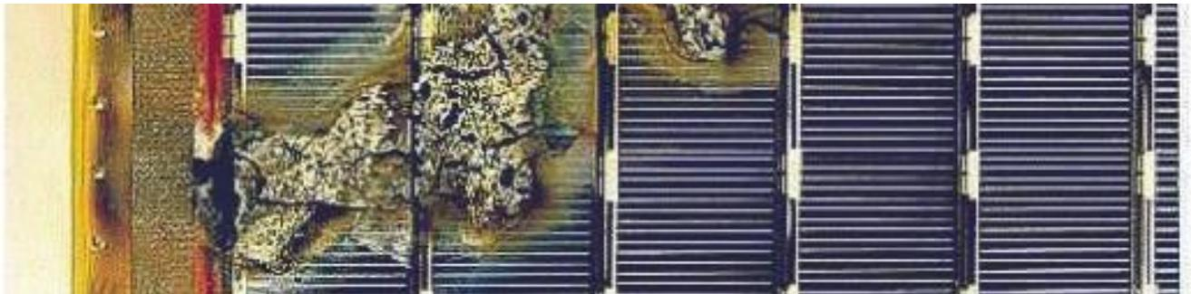
Fig 1. Example of arc damage sustained on a solar array (ESA EURECA)[3]
