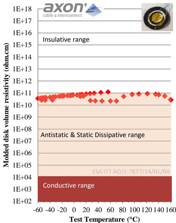
Fig 5. Volume resistivity as function of temperature for an antistatic molded disk specimen W401B1 and measured at 500Vdc. Colored insulation classification range as per ESA and NASA ESD-charging standards [5, 11]
