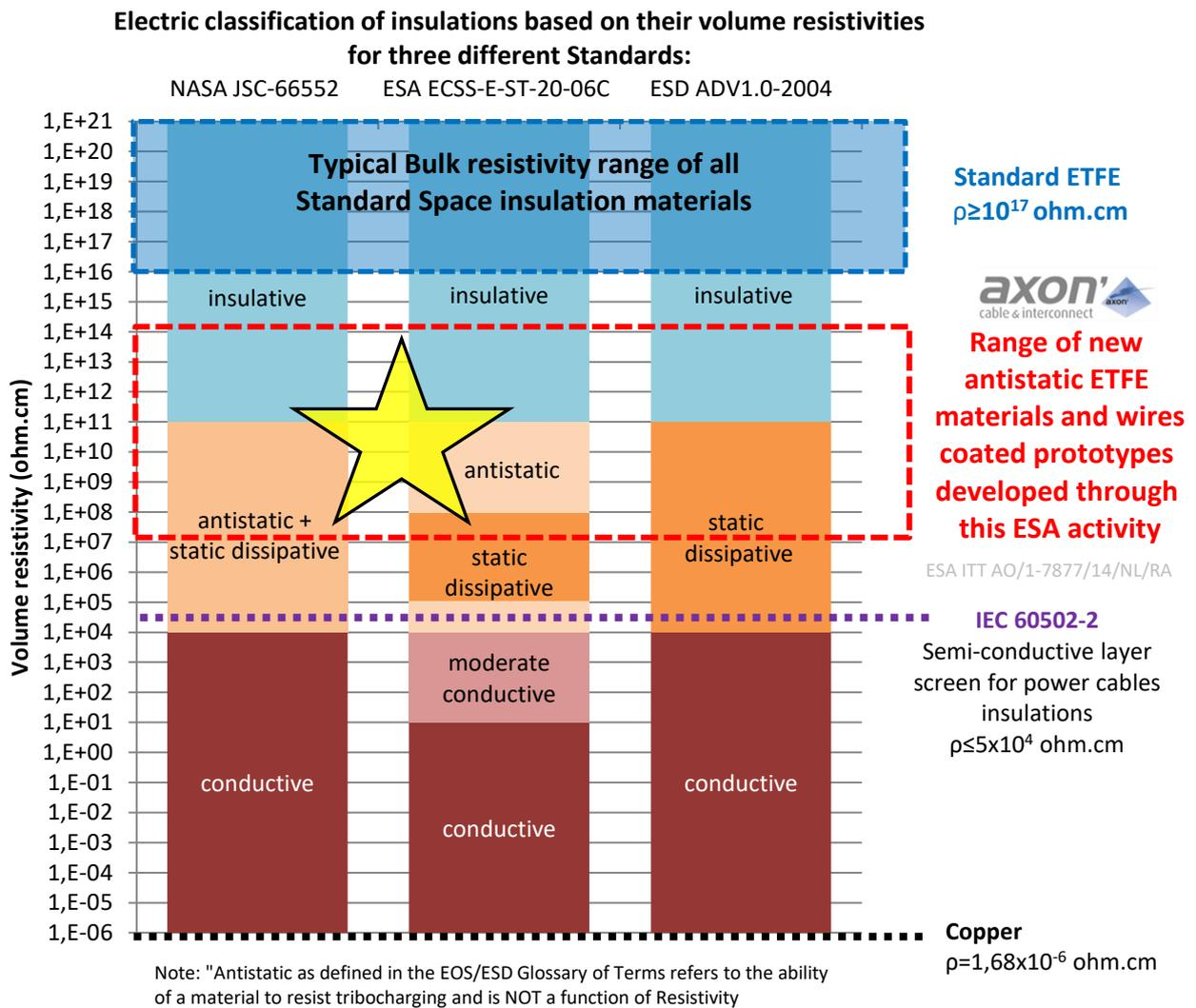
Fig 4. Summary of new modified ETFE-based materials and insulated wires developed through ESA project ITT AO/1-7877/14/NL/RA, as a function of their volume resistivity. Insulation classification ranges based on ESD, ESA and NASA charging standards [5, 11]
