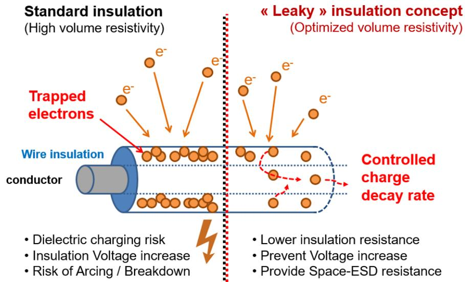
Fig 3. Illustration of the leaky insulation concept explored for the development of new Space ESD resistant wires and cables
