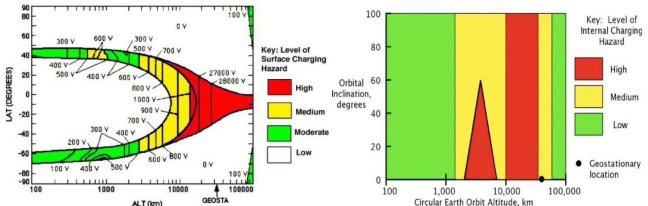
Fig 2. Typical orbits of concerns for surface and internal charging hazards for spacecraft with circular orbits[4]
