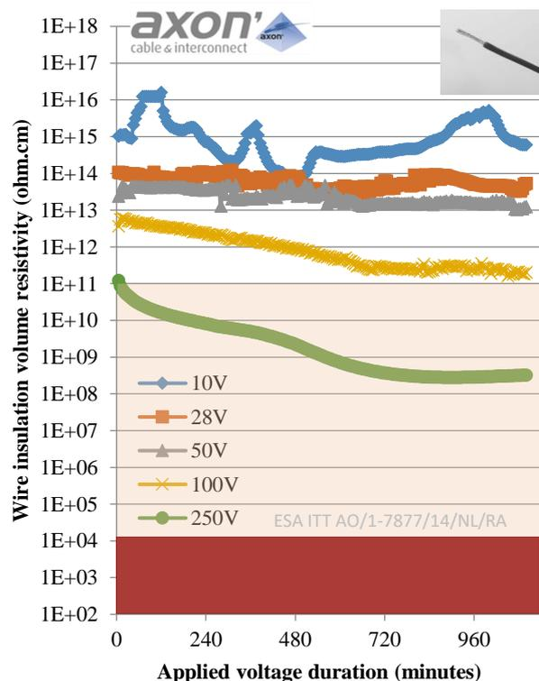
Fig 6. Volume resistivity measurement on the new antistatic modified ETFE wire prototype W4825M1 as function of applied voltage (dc) and testing time duration.
